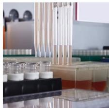
**Span-8 pod** equipped with conductive Liquid Level Sensing (LLS), allows sample volume tracking through Biomek software
