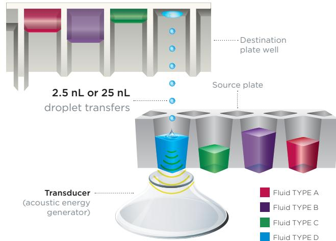
**Acoustic droplet ejection** - The transducer is positioned below the source microplate and emits focused sound energy repeatedly to the meniscus of the fluid to be transferred. A stream of 2.5 or 25 nL droplets (model dependent) is reliably ejected into a well of an inverted destination microplate.
