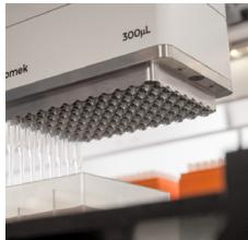
**60, 300 and 1200  $\mu$ L Multichannel heads** with 96 and 384 options for flexible transfer options including individual tip(s), column(s), row(s), patterns
