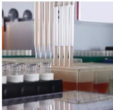
**Span-8 pod** equipped with conductive Liquid Level Sensing (LLS), allows sample volume tracking through Biomek software
