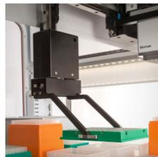
**“High-access” rotating gripper** optimizes access to high-density decks, allows for direct device integrations.
