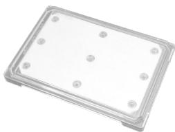
The **MicroClime Environmental Lid** minimizes edge effects and preserves the concentrations of solutions in microplate wells. The novel fluid-absorbing matrix inside the lid can be loaded with water or a compatible solvent to create a vapor barrier, protecting the sample from evaporation and greatly reducing edge effects, and therefore increasing the microplate efficiency by 37%.
