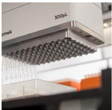
**60, 300 and 1200  $\mu$ L Multichannel heads** with 96 and 384 options for flexible transfer options including individual tip(s), column(s), row(s), patterns
